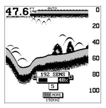
decrease the sensitivity. This typically happens when you wish to see more detail, so an increase in sensitivity is indicated. The procedure to adjust it is the same whether the unit is in the automatic or manual mode.
